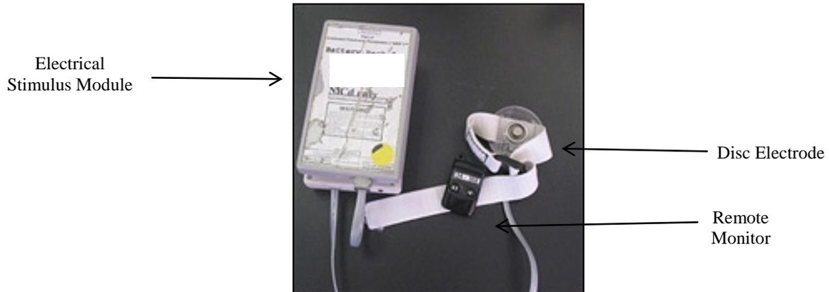
Figure 1: GED Electrical Stimulus Generation Module and Remote Monitor
