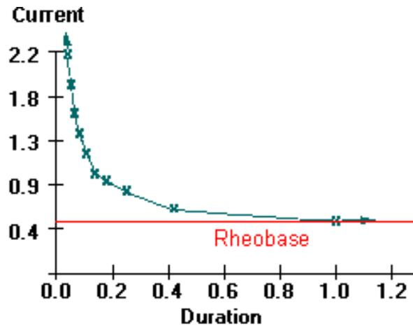
Figure 3: An Example of a Strength-Duration Curve - The Rheobase is the minimum current necessary to elicit a nerve response (e.g., a feeling of paresthesia), at a given pulse width
